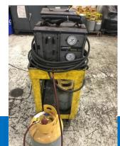
**Refrigerant** Is removed by 608 certified Type I Technician and sent to an EPA certified reclaimer
