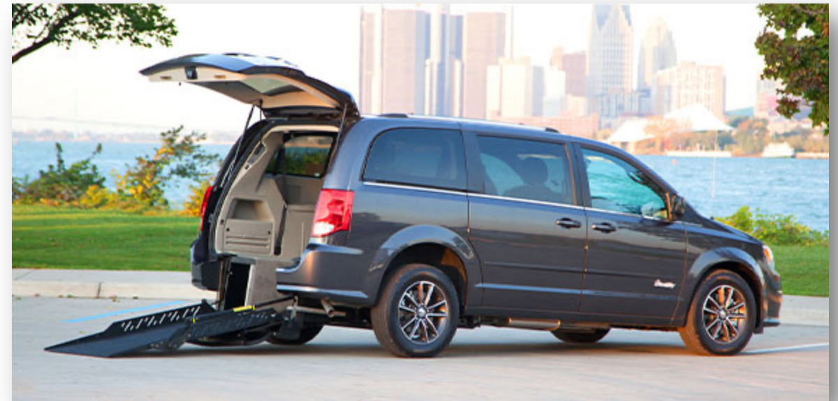
Rear-Entry Lowered-Floor Minivan
